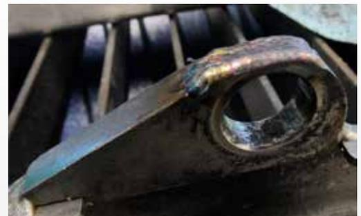
In the fillet welding it is possible the use of Multitack which allows to achieve excellent results. The weld remains white and without any oxidation, thus prevents the acid treatments which often must be applied post welding.
