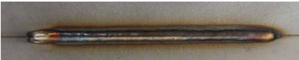
TIG DC continuous fillet weld without additional material
